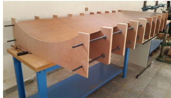
Figure 2.3: Construction of the first PTC from wood
