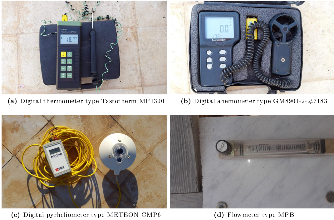
Figure 3.1: The photos of the different measuring devices used during the experiment
