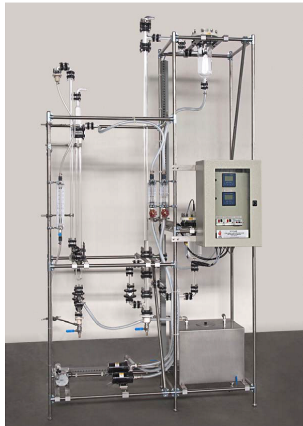
Figure 2.1: Wetted wall gas absorption column.
