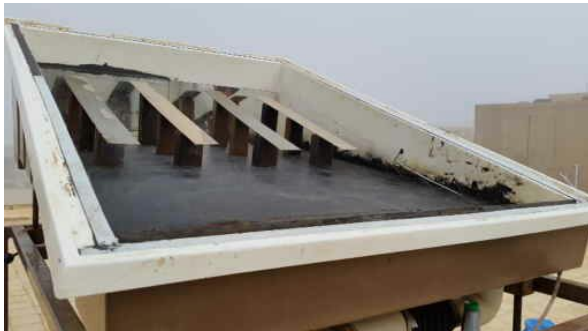
Figure 2.2: Modified solar still with Radiating Surfaces inside the basin
