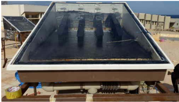
Figure 2.1: Modified solar still with radiating surface and convex lenses on the cover glass
