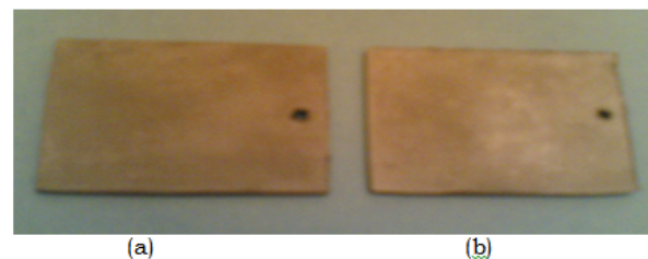
Figure 3.1: The shape of the sample after plating at T=80°C, pH=6.5: (a) No light, (b) Light.
