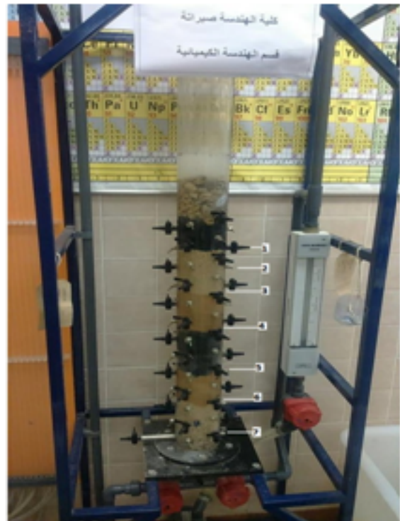
Figure 4.5: Arrangement set of filter media in the column filter design
