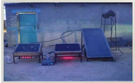
Figure 2.5: Tilted wick and basin type solar still with solar collector.
