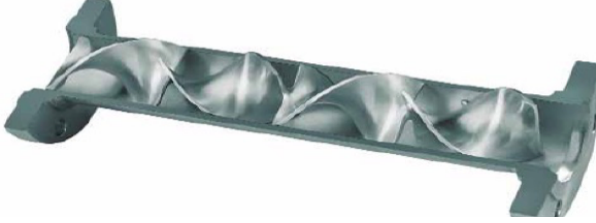
Figure 1.1: The structure of Kenics static mixer
